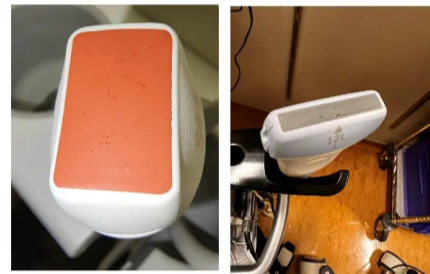
Figure 2. Gouge marks on ultrasound probes indicate contact between the transducer head and needle during percutaneous procedures.
